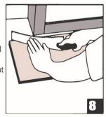
The gap between the bottom of a door and the vinyl flooring should be 1 cm height. To trim door frames, turn a plank upside down.
