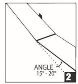
Insert 2nd plank's end tongue to 1st plank's end groove at an angle of 15° to 20°.
