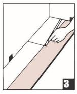
For the last plank of a row, flip a full plank to its under side and place beside the row.
