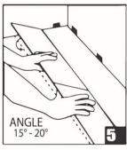
To start second row, assemble your entire row on the subfloor before attaching it to the first row.
